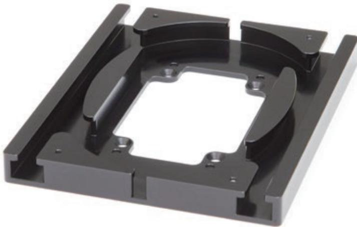
The model 200-TRAY is a machined aluminum fiber management tray that can be mounted directly to a 203, 205, or 207 LaserMount. Wide radius with lipped edges contain the fiber without the need for clips or ties. The tray can also be used with the 200-C cover.
